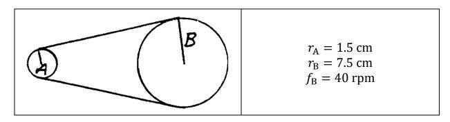
a. Calculate the frequency of the smaller wheel in revolutions per minute.
