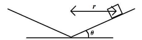
4. E: Use Newton's second law of motion to obtain an equation for the <u>speed</u> of a <u>fast moving car</u> moving at an angle  $\theta$  to the horizontal in circular motion on a banked/angled road with surface friction. Your answer should be in terms of the radius of the track r, the angle of the banked road  $\theta$ , the coefficient of friction  $\mu$ , and the acceleration from gravity g.
