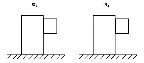
b. Determine an equation for the minimum pushing force in which  $m_2$  does not slide down.
