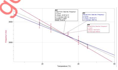
The gradients for the worst fit lines are -35.48 and -50.97, so the uncertainty for the best fit line is  $-15.49 \approx -20$ . Thus, the gradient of the best fit line is -40Hz $\pm -20$ .
